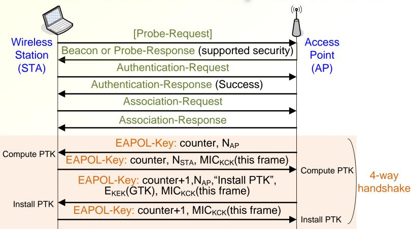
PMK = key derived from Passphrase counter = replay prevention, reset for new PMK PRF = pseudo-random function PTK = PRF(PMK,MACaddr<sub>AP</sub>,MACaddr<sub>STA</sub>,N<sub>AP</sub>,N<sub>STA</sub>) KCK, KEK = parts of PTK MIC = message integrity check, a MAC
