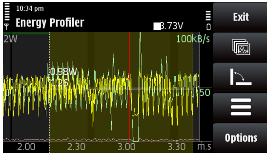
Figure 4: Power Consumption for Bursty Traffic at 50KBps Data Rate
